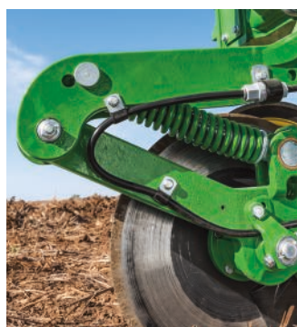
Frame mounted fertilizer opener (sold separately)
